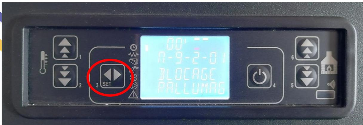
APPUYER SUR LE BOUTON N°5 POUR ALLER JUSQU'À M-9-2-05 ASP FUME PRECHARGE
